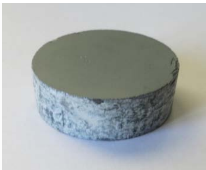
Figure 4: Photo of Briquette Compacted from Ultra Dispersed \text{Si}_{0.7}\text{Ge}_{0.3}+\text{P}_{0.5} Alloy Powder at 1300°C
