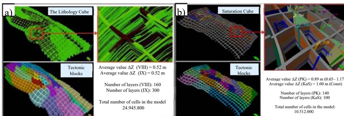
Figure 3: Geometric Parameters of the 3D Grid of Layers VIII and IX (a) and PF and KaF (b)
